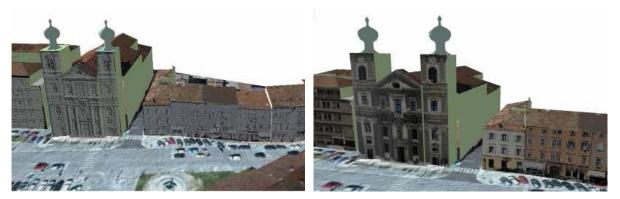
Figure 37: Terrestrial laser scans of the building facades (left) and terrestrial ortho-photos wrapped on the facades (right)
