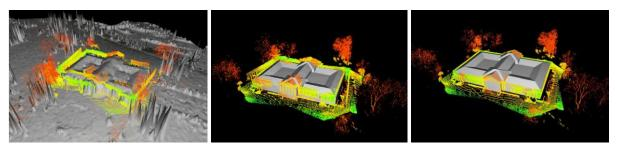
Figure 36: Super-imposition of directly georeferenced terrestrial laser scanner data and aerial LIDAR (left) and virtual city model (centre) with result after alignment (right)
