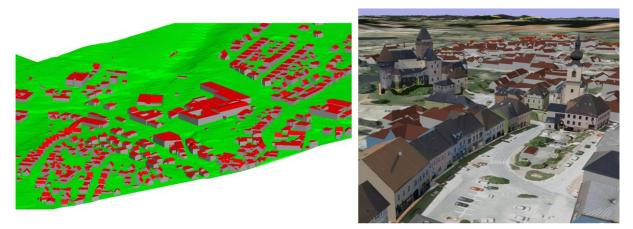
Figure 32: Rendered city model correctly intersected with a DTM triangulation (left); 3D city model with manually applied textures from terrestrial and airborne images (right)
