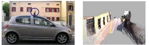
Figure 34: Vehicle with camera (left); Dense 3D reconstruction (right)
