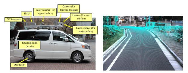
Figure 35: System configuration of MMS (TYPE-S) (left); MMS measurement data (right)
