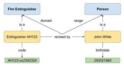
Figure 54: Example of graphical representation of an ontology.
