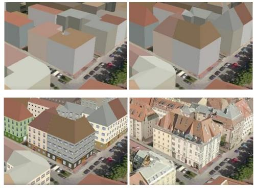
Figure 44: Example of different LoDs in the BLOM3D<sup>™</sup> [78]. BlomLOD1<sup>™</sup> (upper left), BlomLOD<sup>™</sup> (upper right), BlomLOD3<sup>™</sup> (bottom left), BlomLOD4<sup>™</sup> (bottom right)
