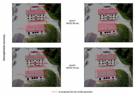
Figure 30: Residuals at image plan and visual overlay accuracy direct vs. integrated geo-referencing solution
